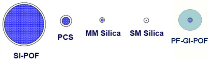
Fig. 2.1. Relative comparison of diameters in different kinds of fibers. SI-POF=step-index polymeric optical fiber; PCS=plastic cladding silica fiber; MM Silica=multimode silica fiber; SM silica=single mode silica fiber; PF-GI-POF=perflorinated graded-index POF. The light color represents the cladding and dark color the core.
