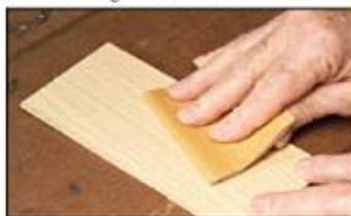
Sanding the surface before scrolling makes finishing easier in the long run.
