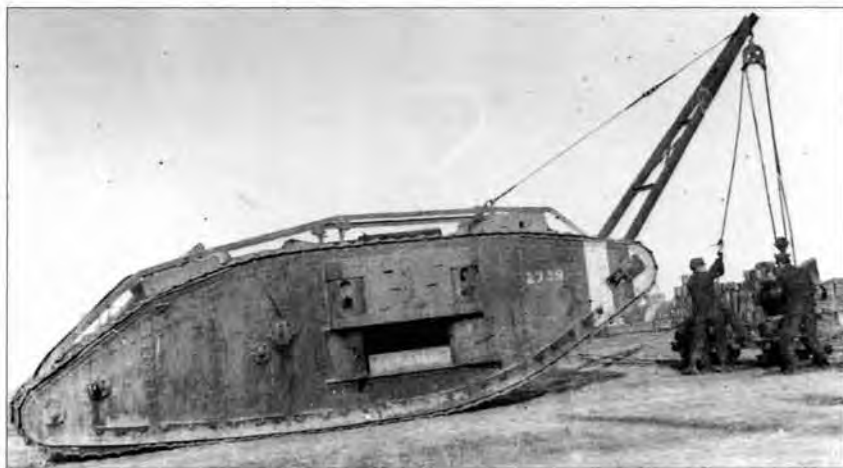
A Mark IV female fitted with a portable tank crane lifts heavy items onto light railway wagons, probably at the depot in France. The jib is secured to the back of the cab and employs a manual chain hoist.
