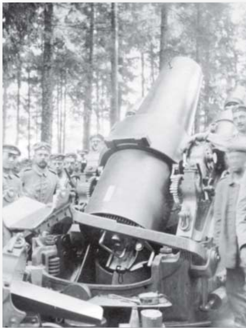
Fielded in 1897, the 30.5cm Beta-Gerät mortar was the German Army's first siege gun. Simple to operate and reliable, the mortar was employed throughout the war on both the Western and Eastern fronts. (M. Romanych)
