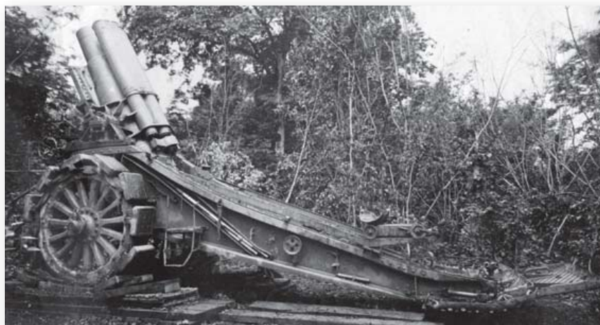
The 28cm L/12 i.R. howitzer was essentially a large version of the heavy artillery's 21 cm howitzer. Only one prototype howitzer was built and fielded in 1914 with SKM Battery 7. (M. Rupp)
