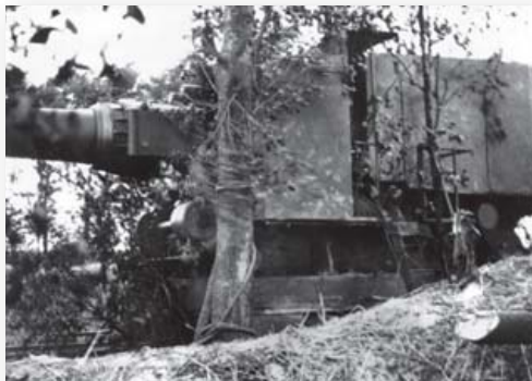
By 1916, Gamma howitzers were fitted with armored cabs to protect the crew in the event that the gun was shelled by enemy counter-battery fire. This howitzer is emplaced near Biache-Saint-Vaast in October 1917. (M. Romanych)
