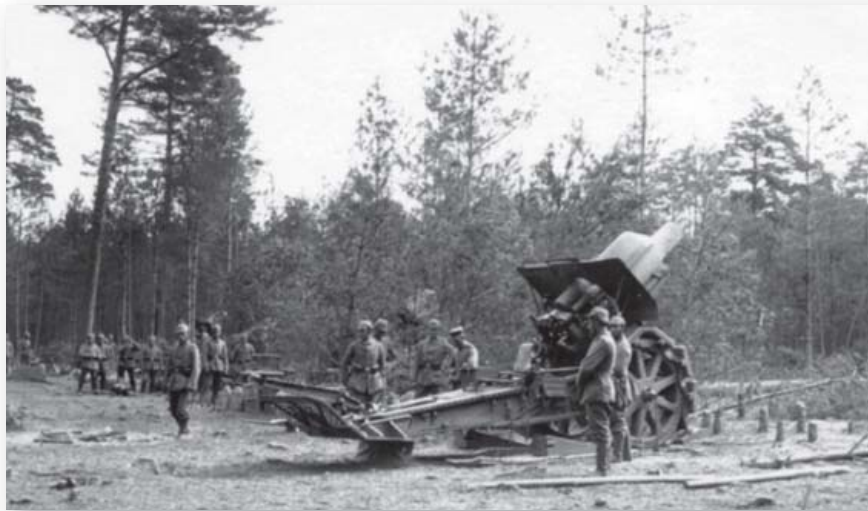
A battery of 21cm howitzers prepared for action. Both Belgium and France designed their fortifications to withstand hits by 21cm projectiles, not realizing that the German Army would develop larger caliber mobile siege guns. (M. Romanych)
