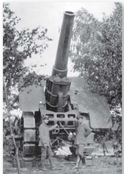
The German Army's first large-caliber siege gun mounted on a wheeled carriage was the 30.5cm Beta i.R. howitzer. The design of the howitzer incorporated features from both the 28cm L/12 i.R. and L/14 i.R. howitzers. (M. Romanych)
